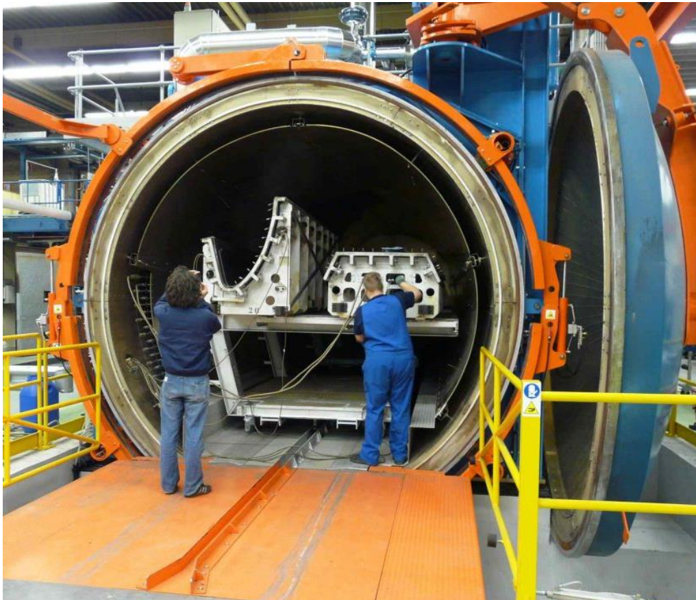
Figure 32 Large autoclave used in aircraft manufacturing
