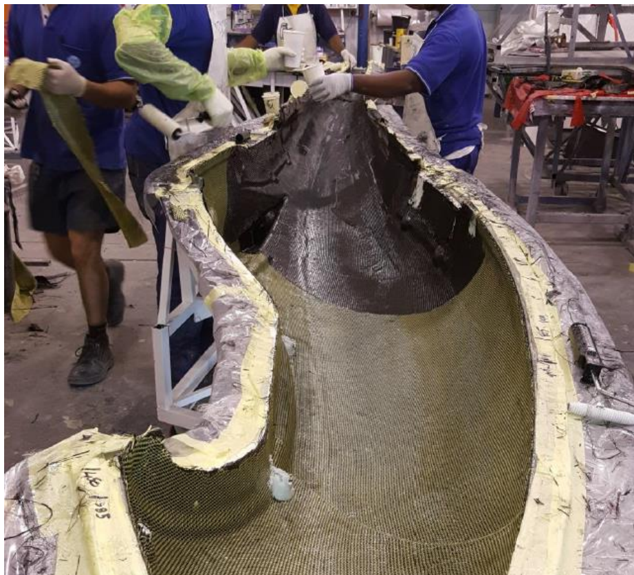
Figure 18 Open moulding process used for constructing the JS3's fuselage
